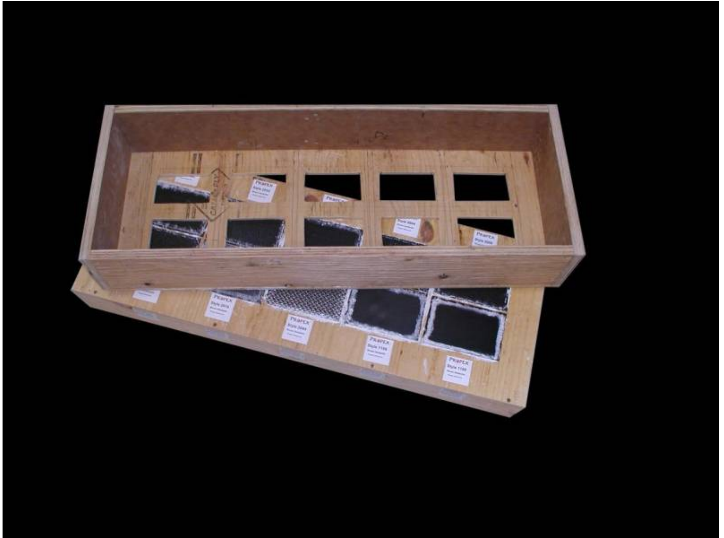
Figure 7: Top and bottom parts of the box test.
