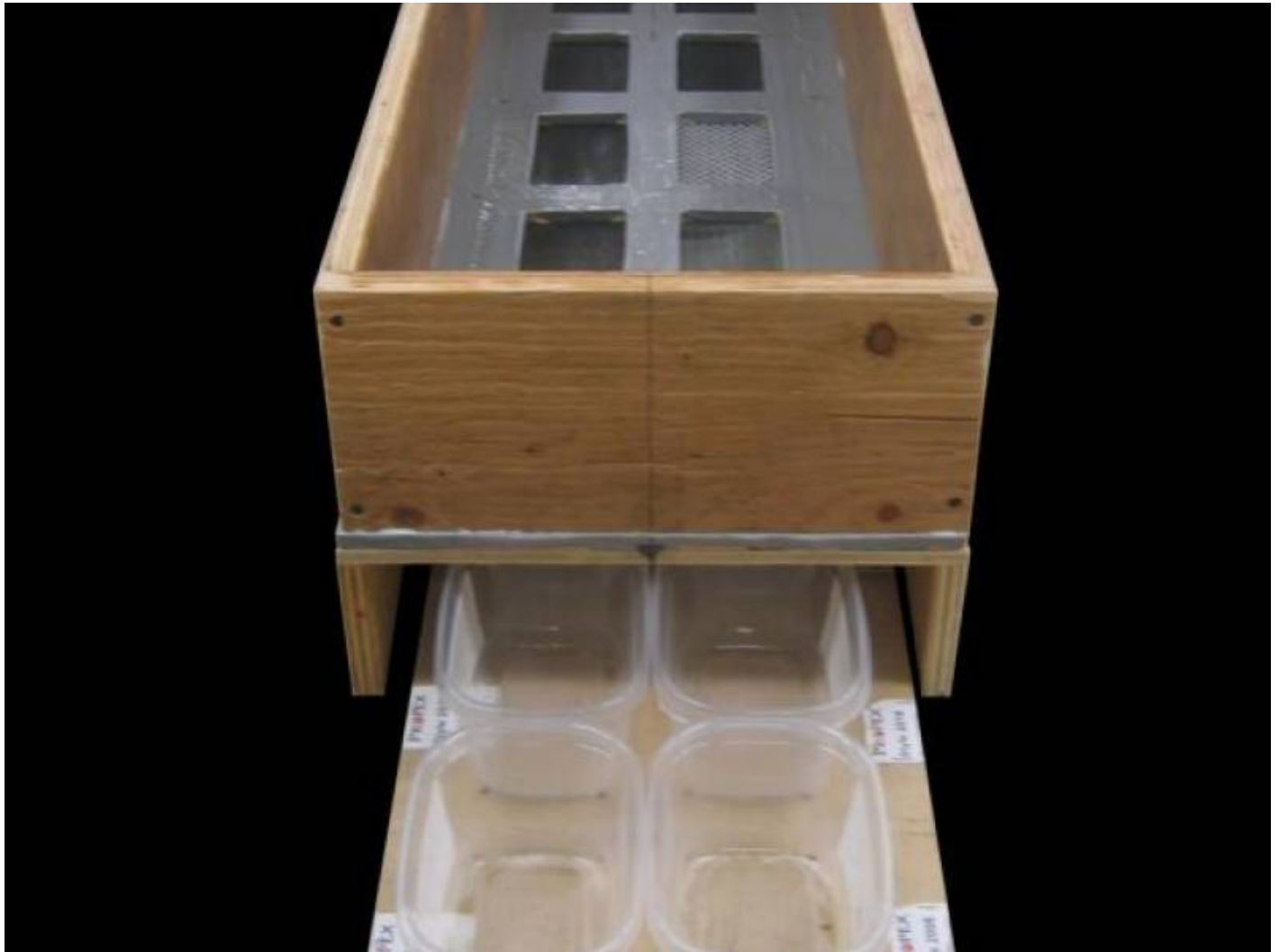
Figure 8: Box made for Box Test using normal concrete.
