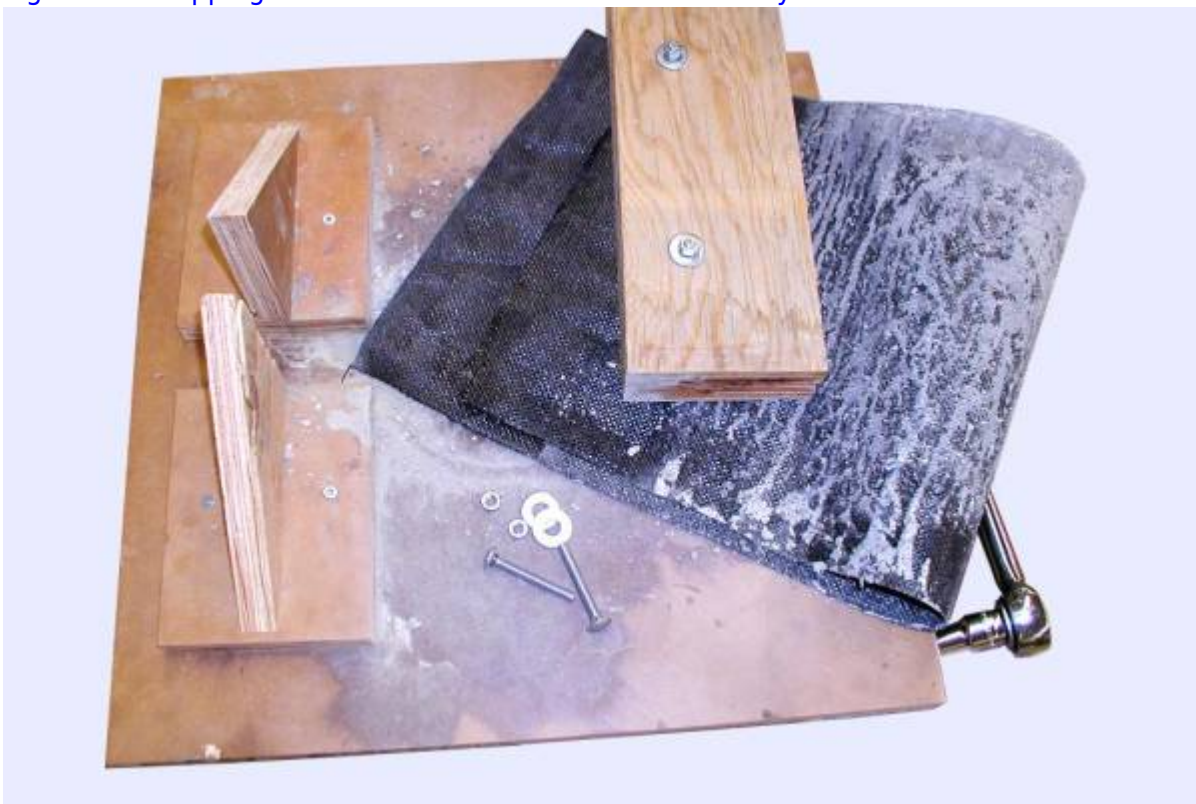
Figure 25: Reusable fabric form parts; the base, sandwich boards, bolts, and the...
