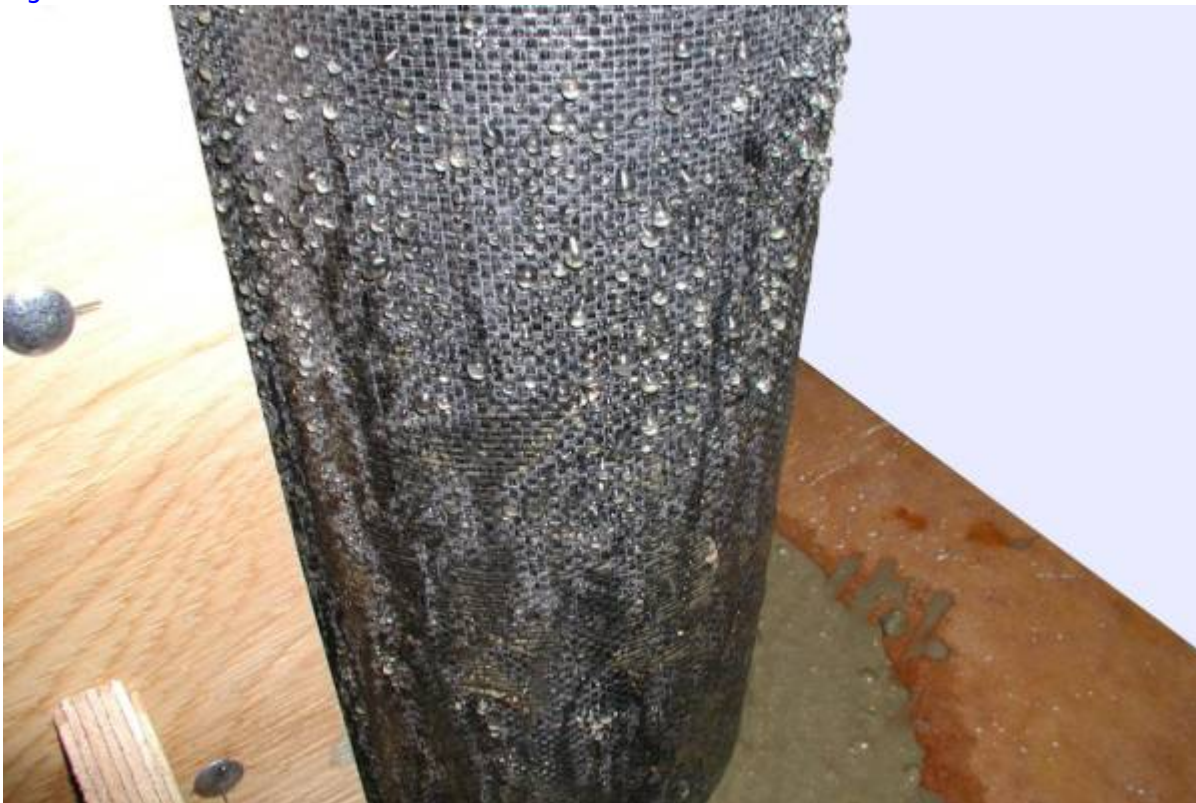
Figure 23: Bleed clear water from the walls of a 152 mm (6 in.) diameter...
