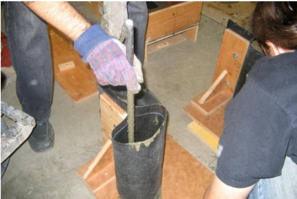
Figure 21: Compacting fresh concrete using the standard rod.
