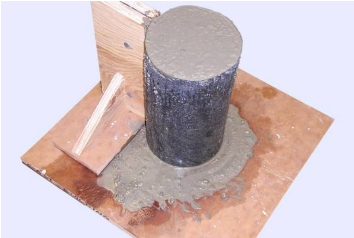
Figure 22: Fabric mold filled with fresh concrete.
