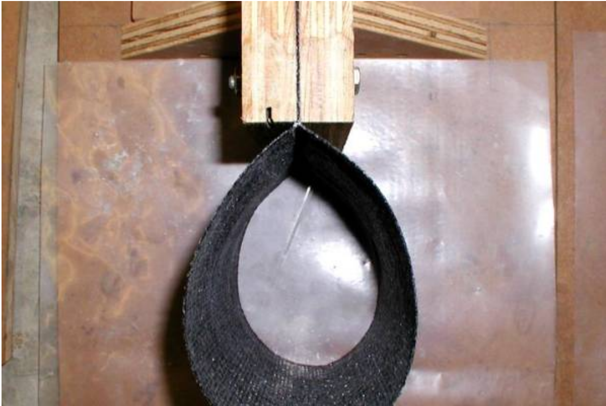
Figure 33: Fabric formwork shown from above.
