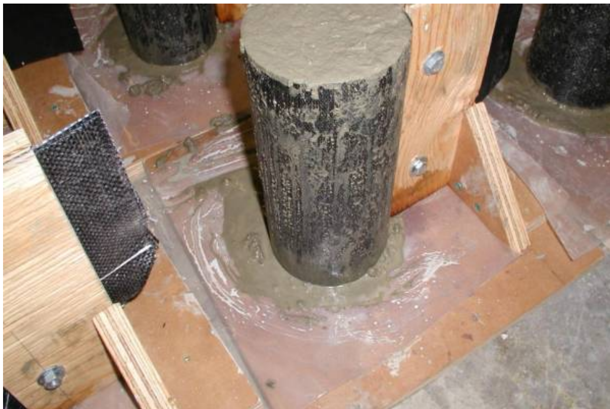
Figure 34: Fabric-formed concrete cylinders.
