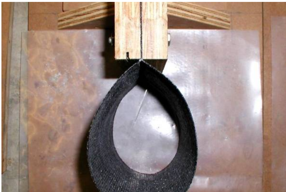
Figure 33: Fabric formwork shown from above.
