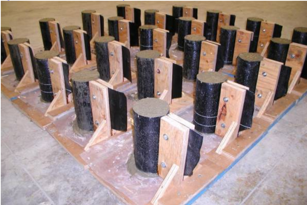
Figure 35: Fabric-formed cylinders after casting.
