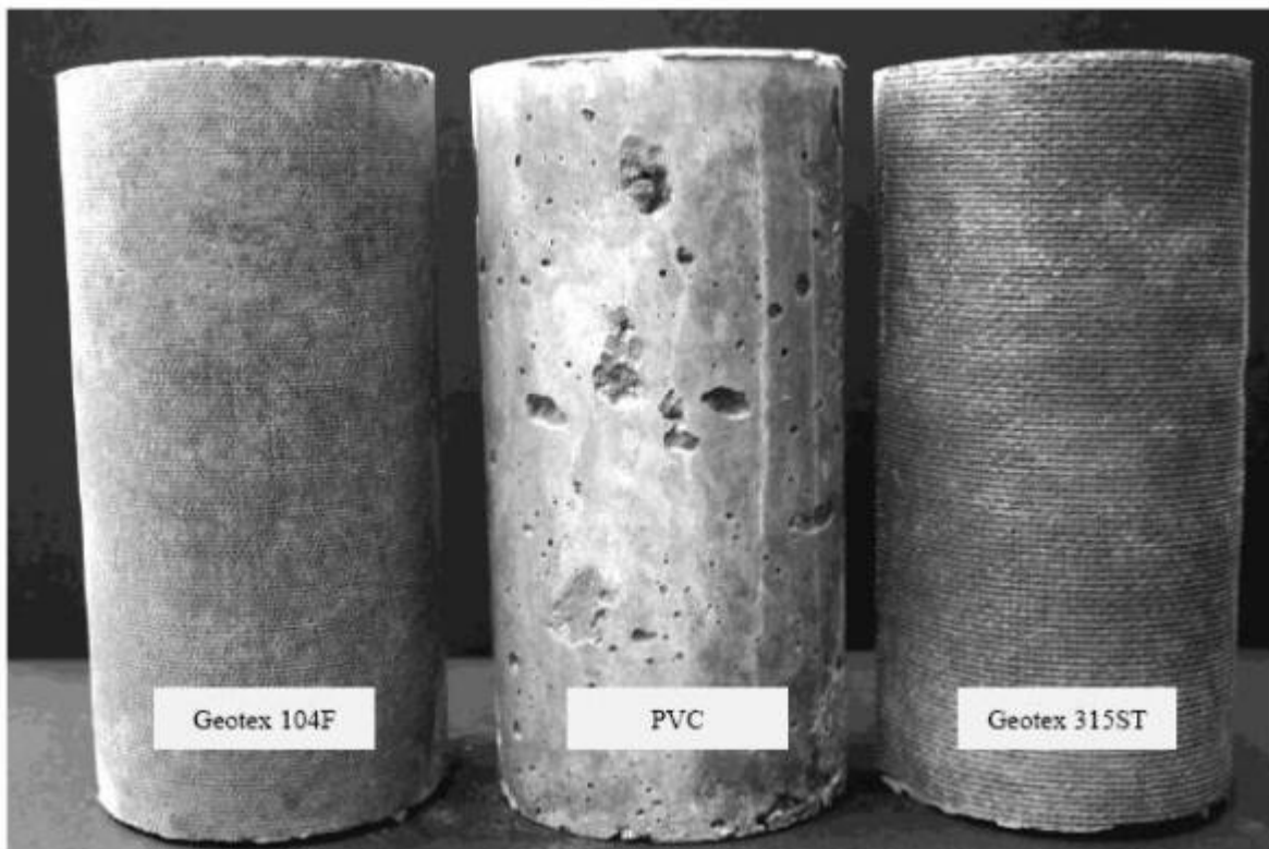
Figure 37: The effect of mold on quality of quality of concrete finish.
