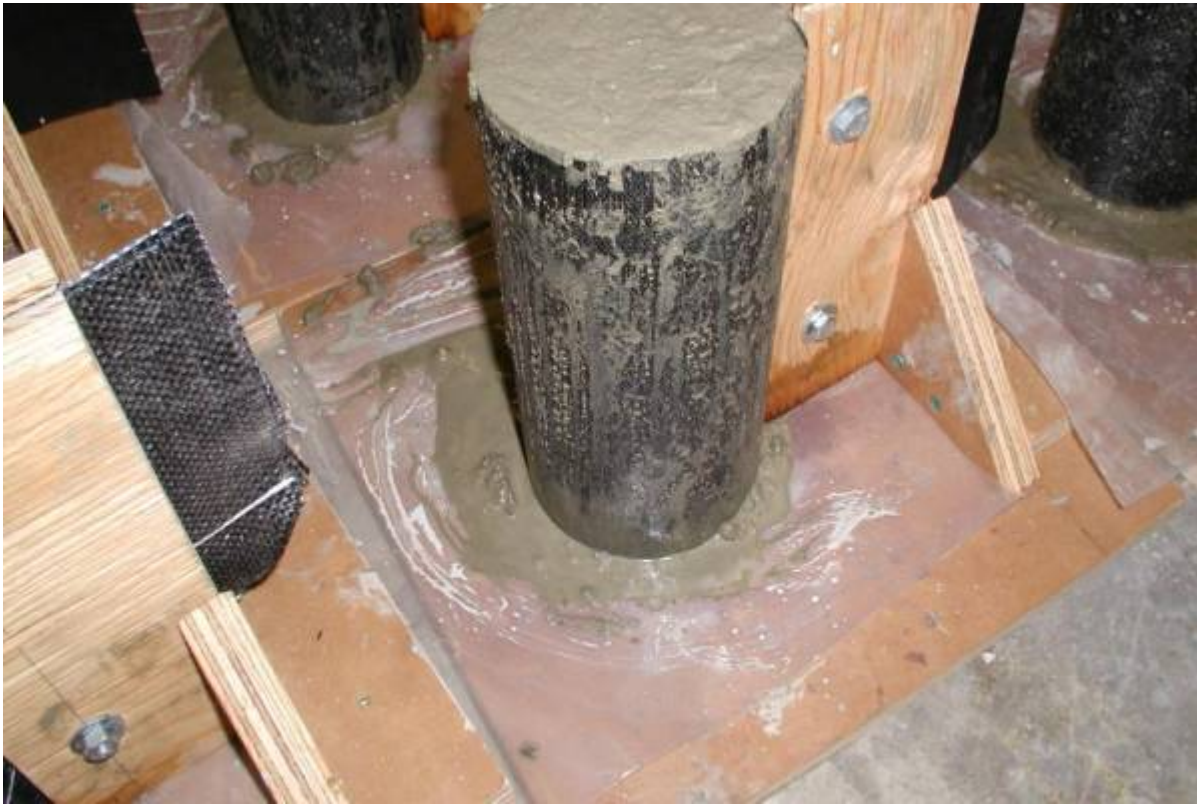
Figure 34: Fabric-formed concrete cylinders.
