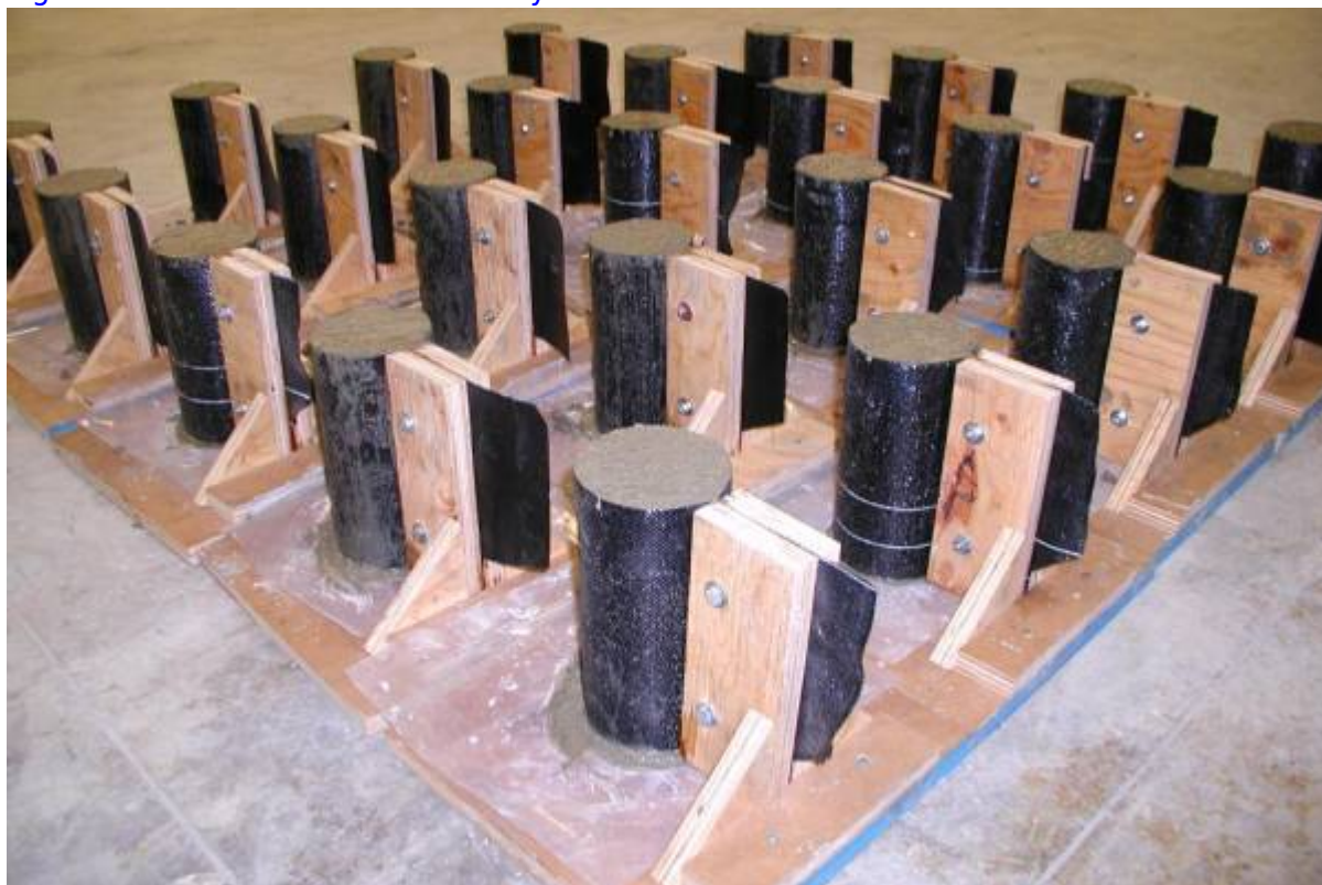
Figure 35: Fabric-formed cylinders after casting.
