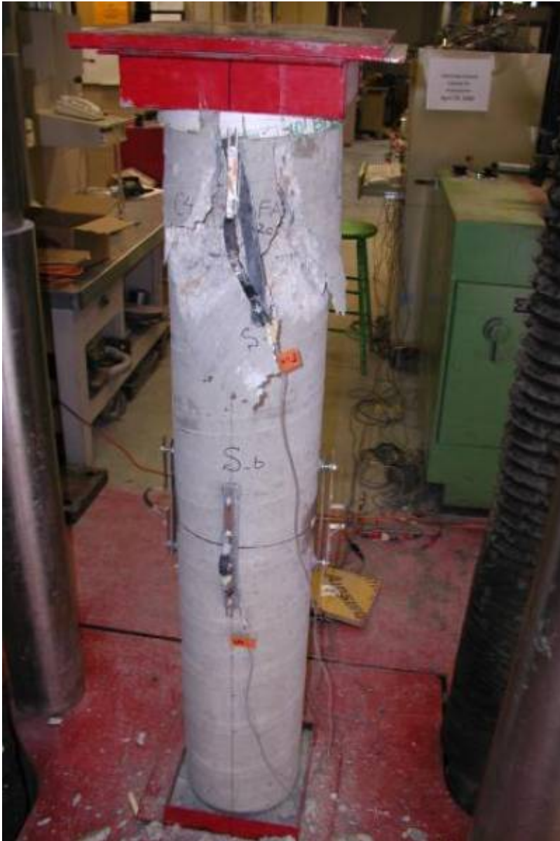
Figure 65: Column CT-FAC after failure.
