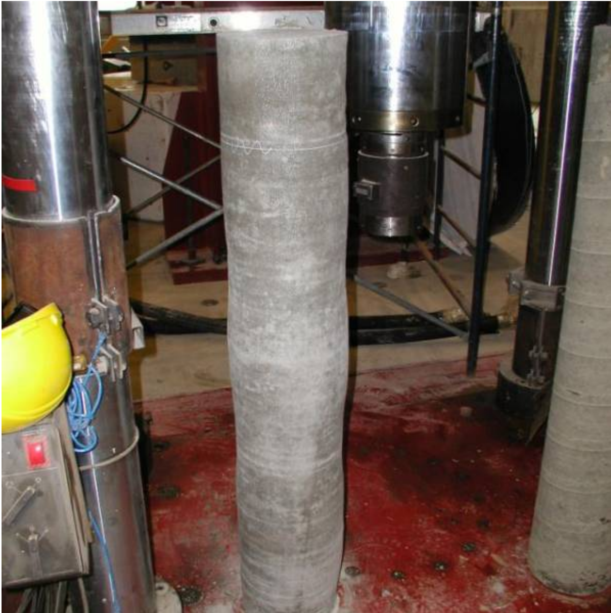
Figure 67: Bulged concrete column.
