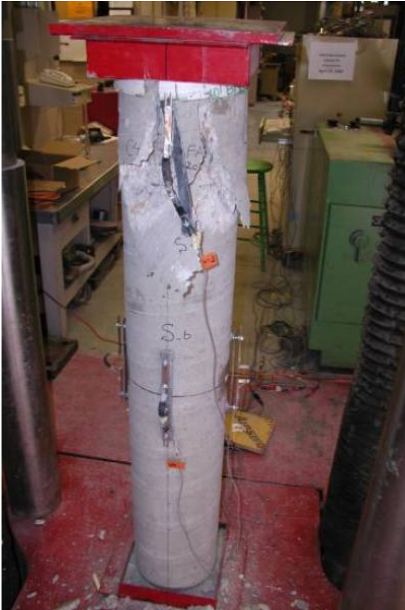
Figure 65: Column CT-FAC after failure.
