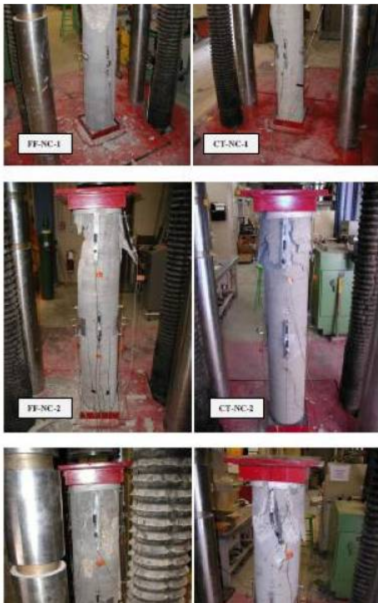
Figure 65: All columns after failure.
