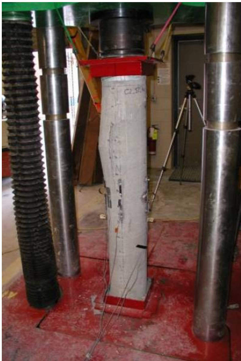
Figure 65: Column CT-NC-1 after failure.
