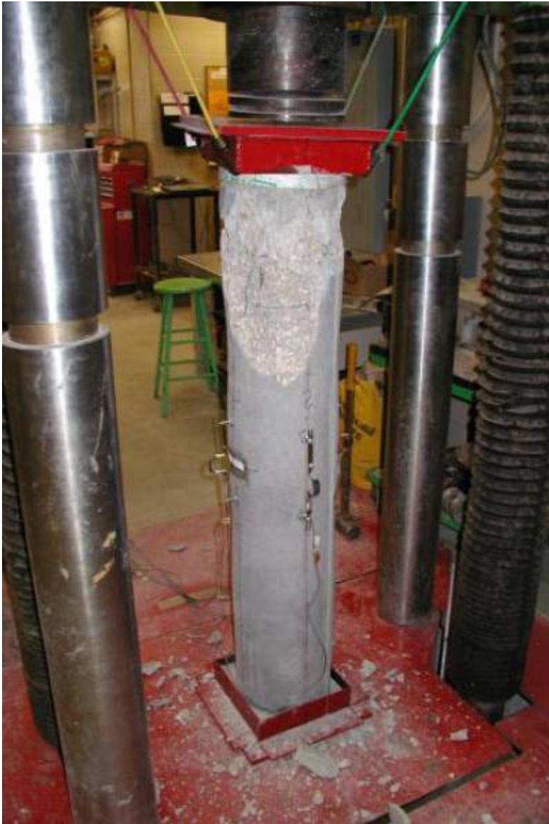
Figure 65: Column FF-NC-1 after failure.
