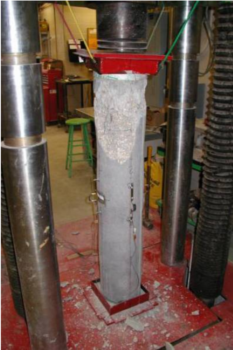
Figure 65: Column FF-NC-1 after failure.
