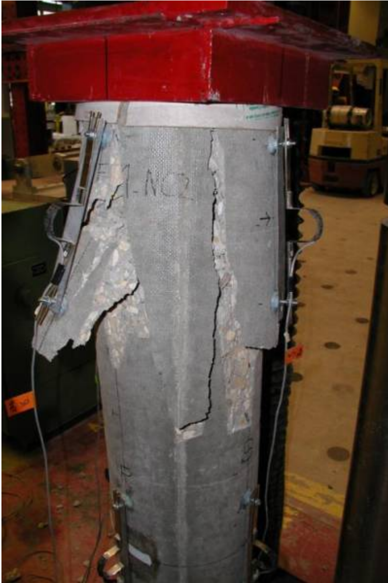
Figure 64: Column FF-NC-2 after failure.
