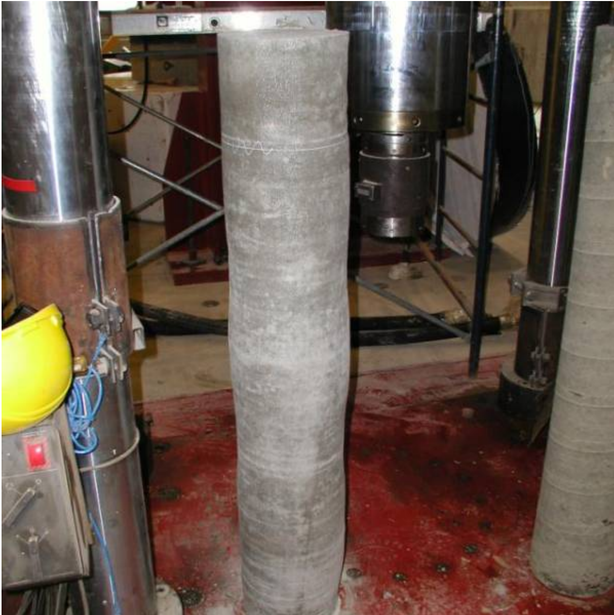
Figure 67: Bulged concrete column.
