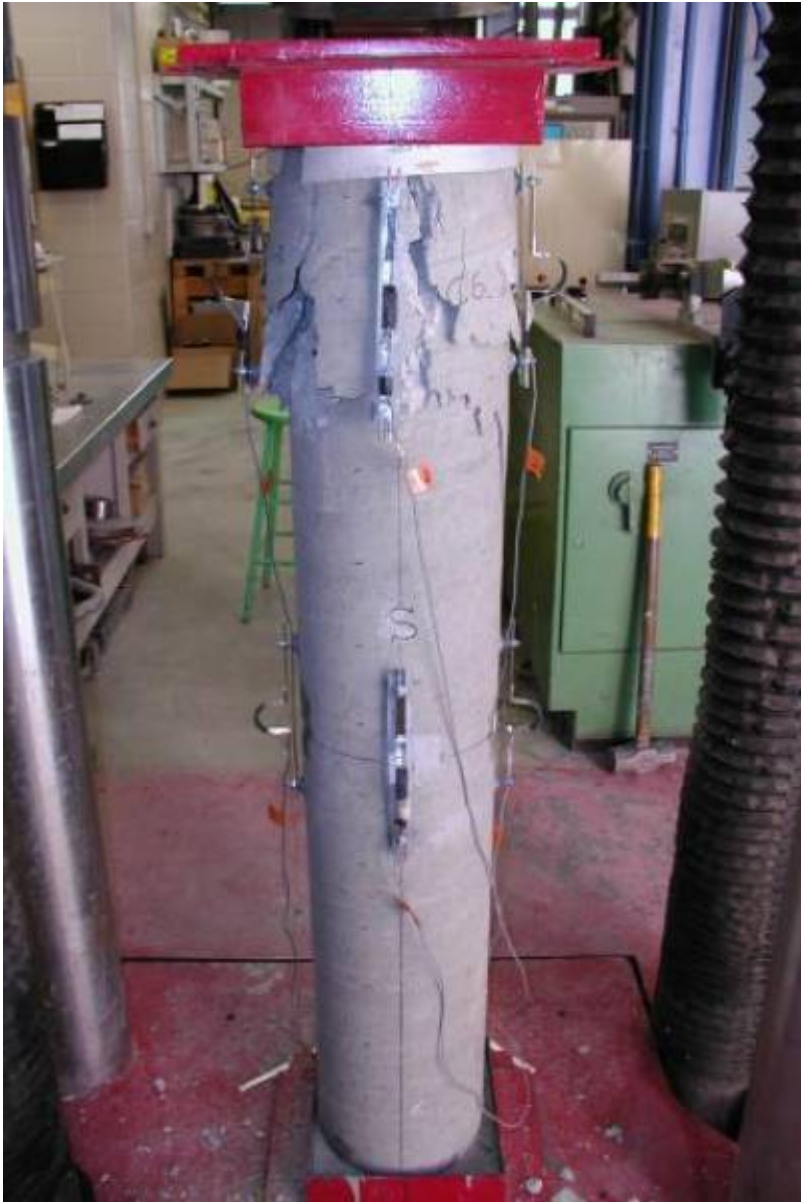
Figure 65: Column CT-NC-2 after failure.
