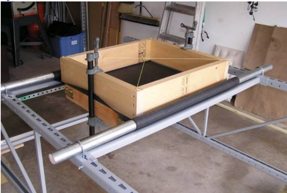
Figure 4: Test Frame with Curb.
