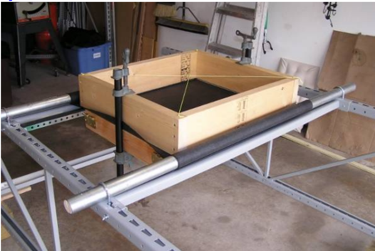
Figure 4: Test Frame with Curb.
