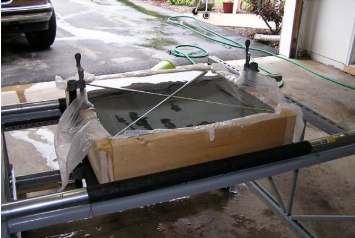
Figure 5: Test Frame with Loaded Fabric.
