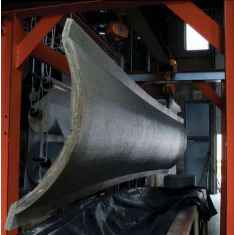
Fig. 35. Removing 3 cm (1.2 in) vault from formwork.
