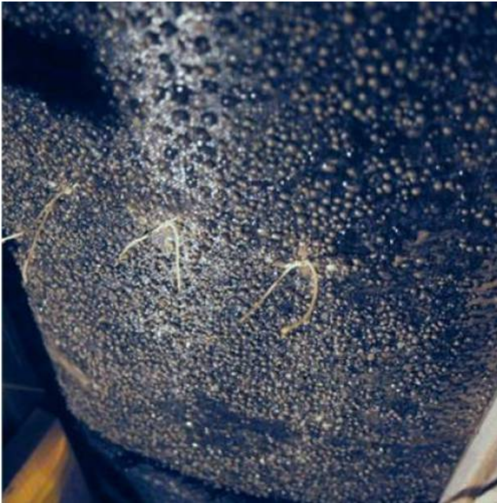
Fig. 12. Filtration of excess water and air bubbles through geotextile fabric.
