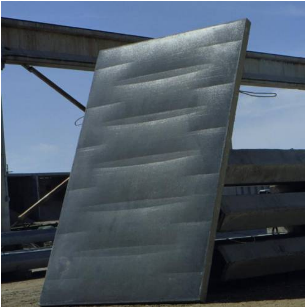
Fig. 10. Completed full scale concrete wall panel.
