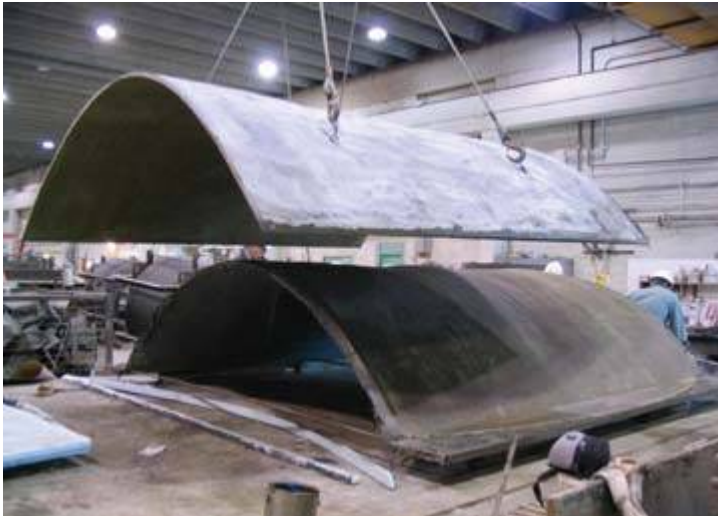
Fig. 23. Step 2- Uniform layer of GFRP is applied.
