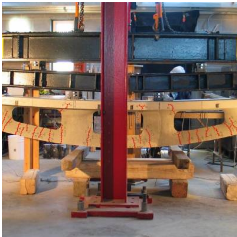
Fig. 15. Testing of variable section concrete truss.
