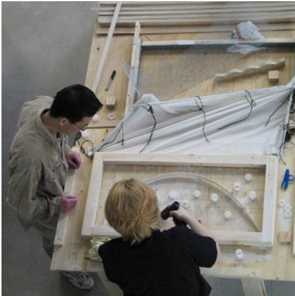
Fig. 1. Model wall panel formwork.
