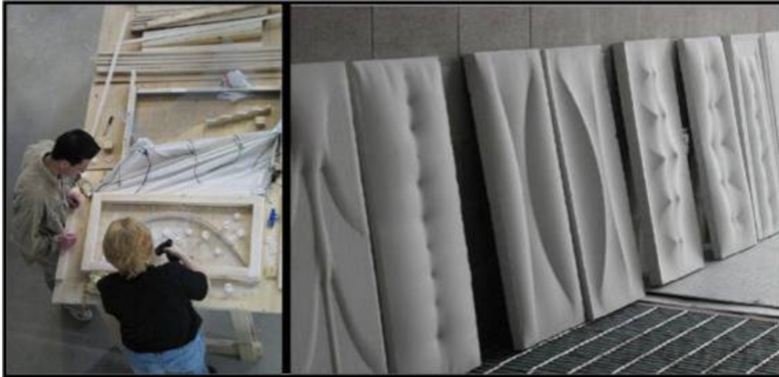
Fig. 1. Model formwork and completed plaster cast.
