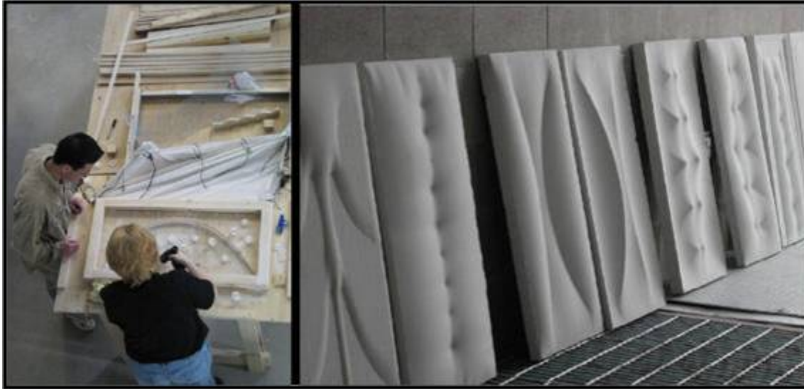
Fig. 1. Model formwork and completed plaster cast.
