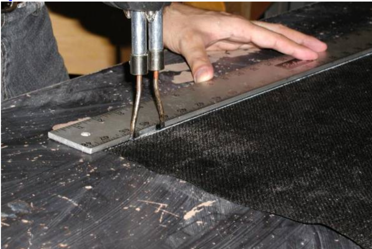
Figure 18: Soldering gun with the blade-shaped tip melting fabric and providing...
