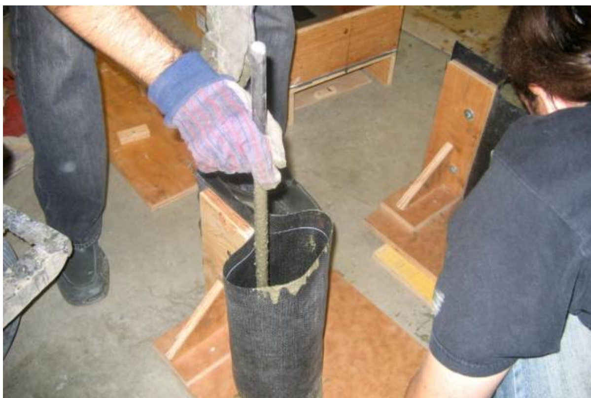
Figure 21: Compacting fresh concrete using the standard rod.
