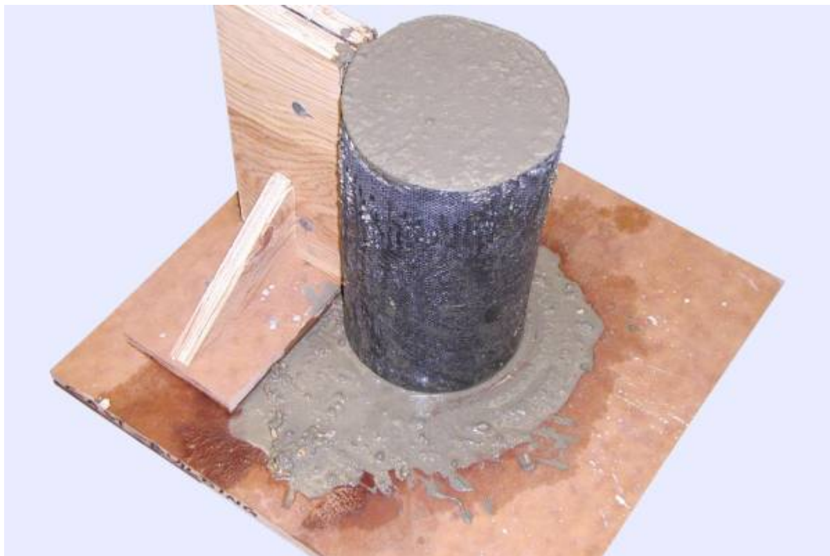
Figure 22: Fabric mold filled with fresh concrete.
