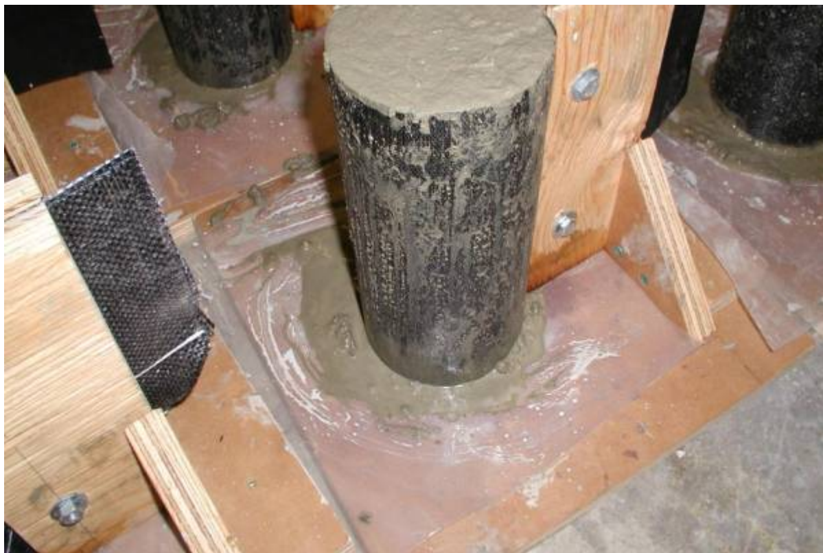
Figure 34: Fabric-formed concrete cylinders.
