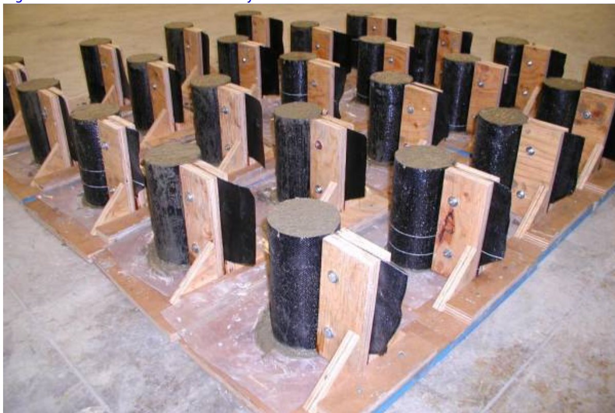
Figure 35: Fabric-formed cylinders after casting.
