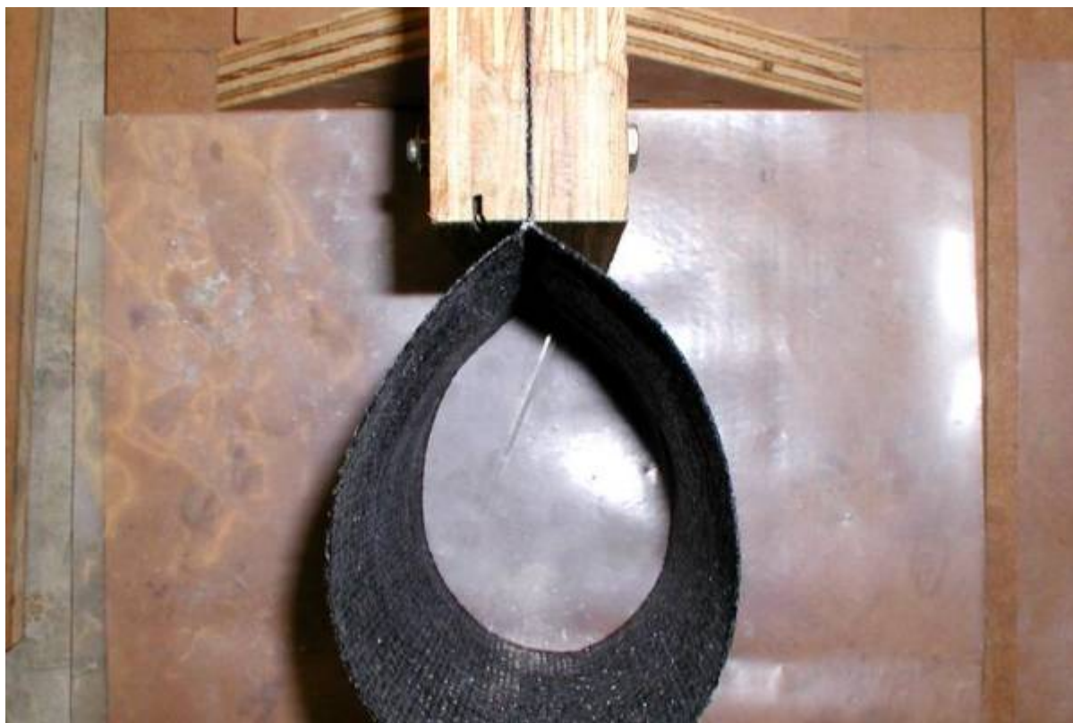
Figure 33: Fabric formwork shown from above.
