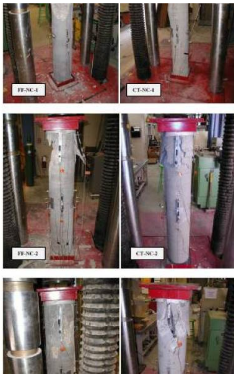
Figure 65: All columns after failure.
