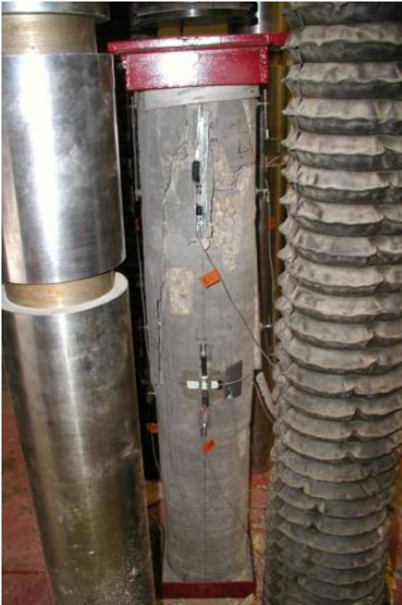
Figure 65: Column FF-FAC after failure.
