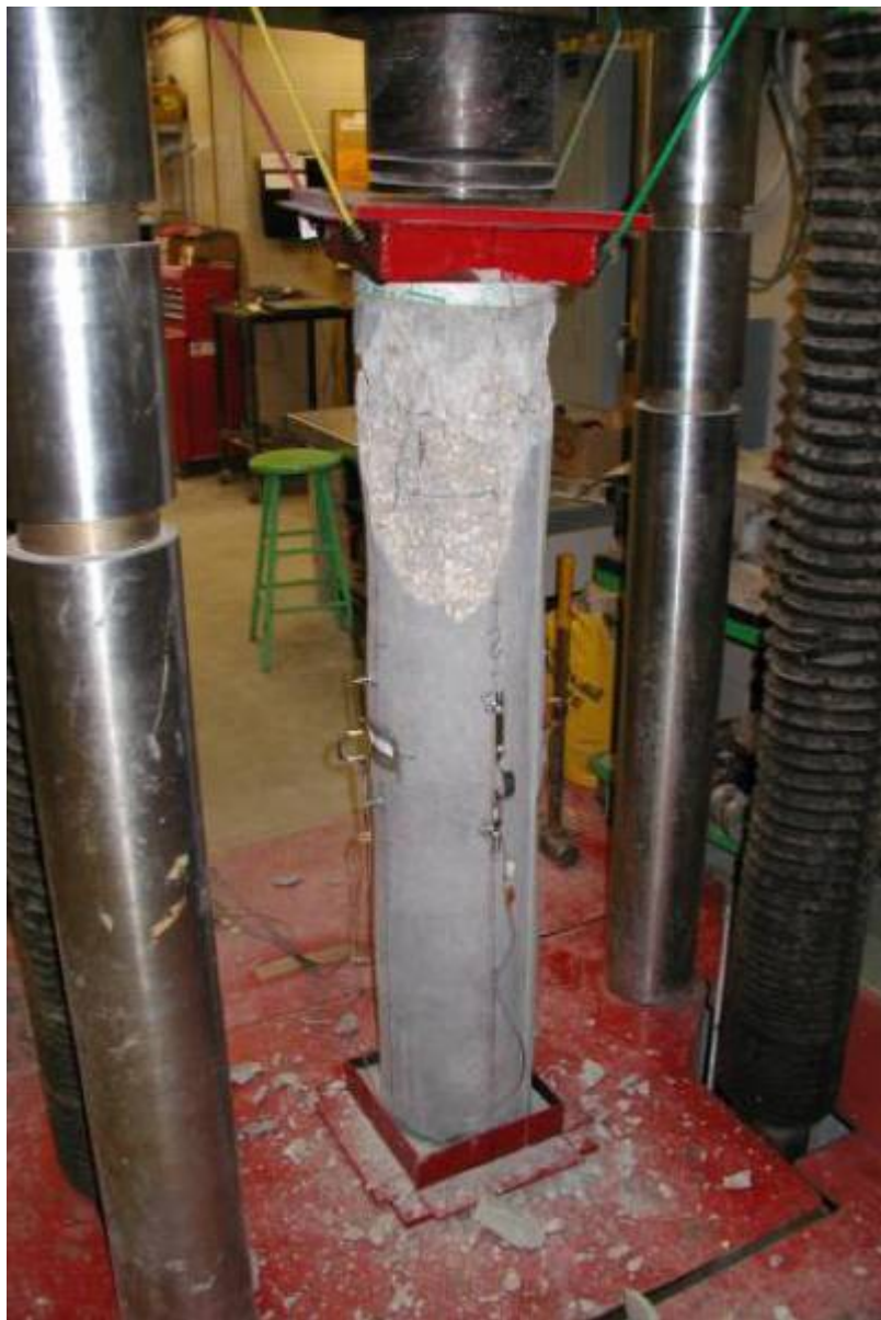
Figure 65: Column FF-NC-1 after failure.
