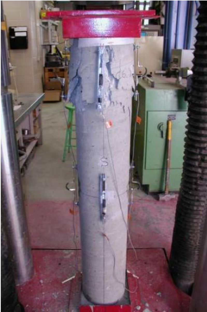
Figure 65: Column CT-NC-2 after failure.
