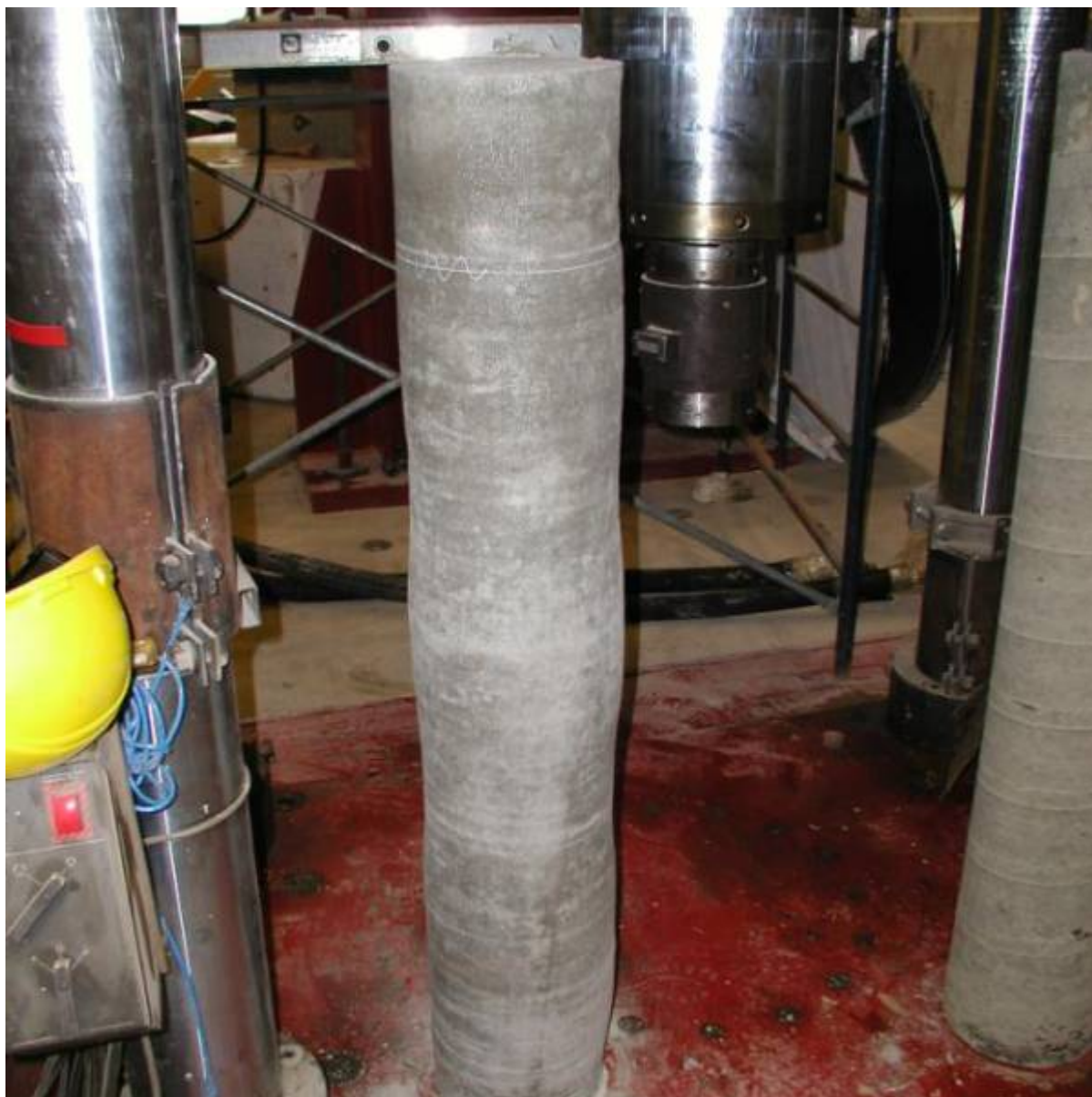
Figure 67: Bulged concrete column.
