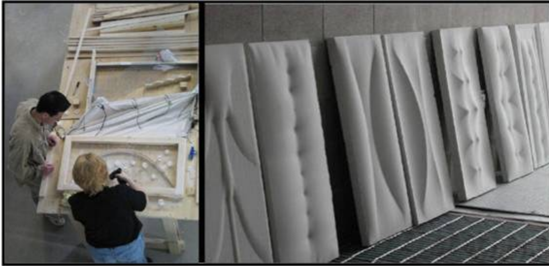
Fig. 1. Model formwork and completed plaster cast.
