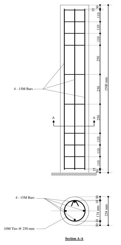
Figure 42: Column reinforcement details
