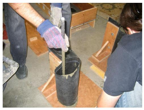
Figure 21: Compacting fresh concrete using the standard rod
