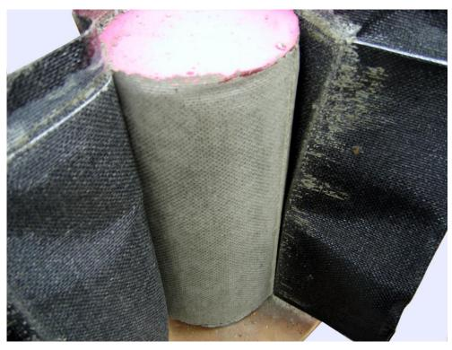
Figure 24: Stripping fabric from a fabric formed concrete cylinder
