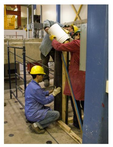
Figure 47: casting of column in fabric formwork
