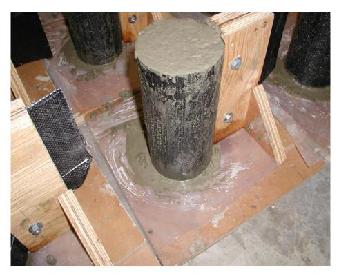
Figure 34: Fabric-formed concrete cylinders
