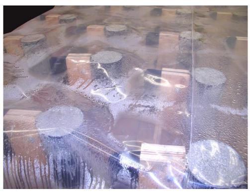
Figure 36: Cylinders curing
