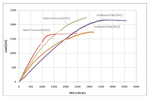
Figure 55: Maximum axial load of fabric-formed versus cardboard-formed steel reinforced concrete columns (Normal and flyash concrete)
