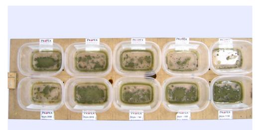
Figure 11: Collected bleed cement/water paste from fabrics tested with normal concrete in the box test
