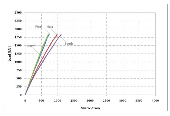
Figure E1: Column FF-NC-1, all pi-gauges
