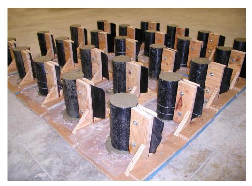
Figure 35: Fabric-formed cylinders after casting
