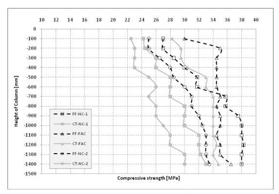
Figure 50: Results from the Rebound tests showing the variation of strength through the height of the columns at the age of 28 days
