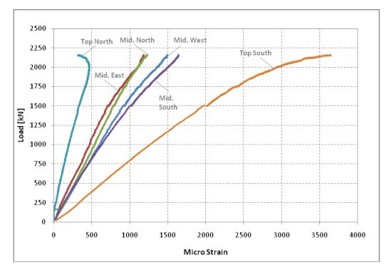
Figure E4: Column CT-FAC, all pi-gauges
