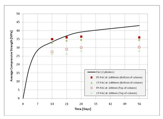
Figure 52: Flyash concrete cylinders compared to Schmidt hammer results (Columns FF-FAC & CT-FAC)
