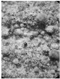
b) Material bled from Geotex 104F showing some flyash beads along with the fine aggregates (mostly cement)
