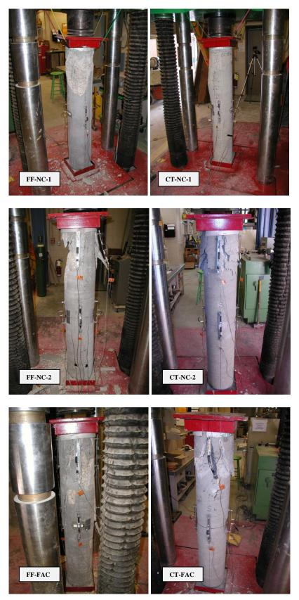
Figure 65: All columns after failure
