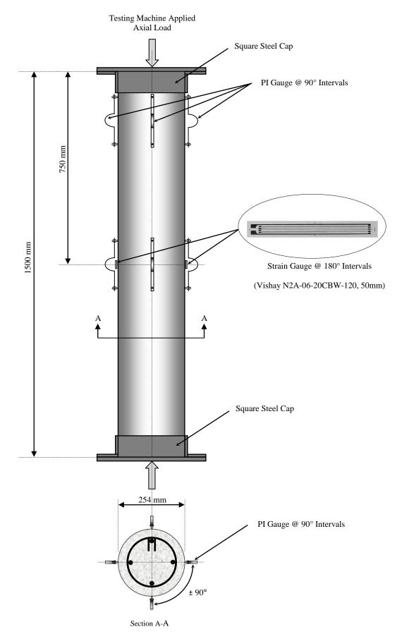
Figure 48: Configuration of the instrumentation of the concrete columns
