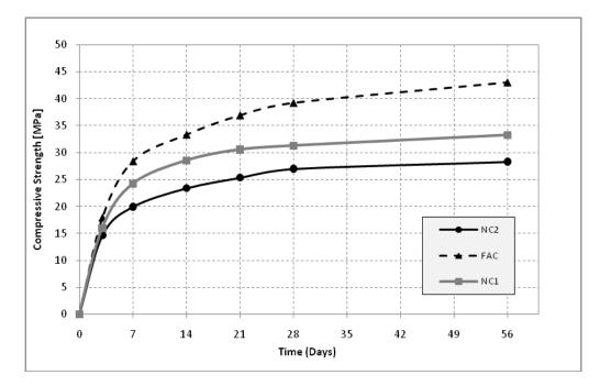
Figure 49: Concrete strength gain with time
