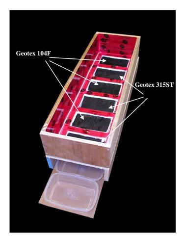
Figure 14: Box made for Box Test 2
