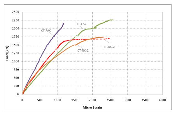
Figure 63: Readings from East pi-gauges at the top of all columns
