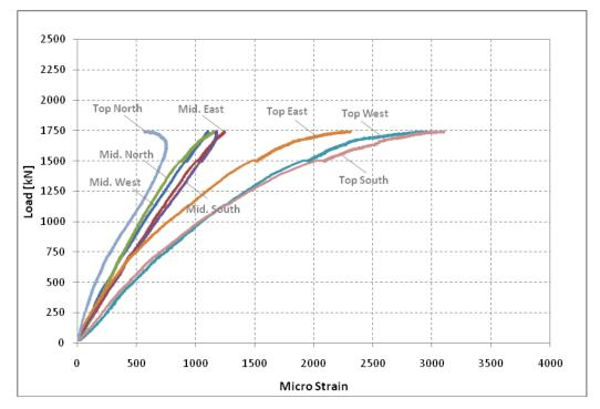
Figure E6: Column CT-NC-2, all pi-gauges
