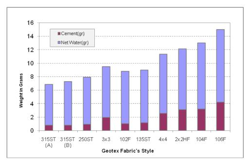
Figure 12: Results from normal concrete box test
