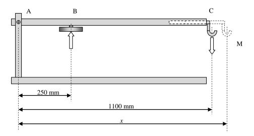
Figure B2: Press apparatus configurations and details
