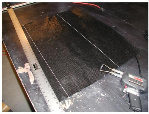
Figure 17: Tools used to cut fabric
