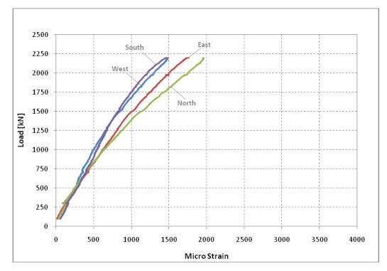
Figure E2: Column CT-NC-1, all pi-gauges
