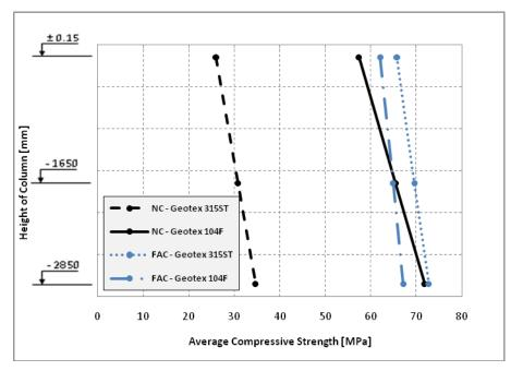
Figure 31: Average rate of strength increase with depth in fabric formed concrete
