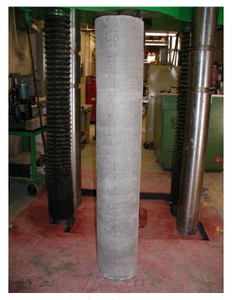
Figure 68: Modified fabric formwork resulting in a straight column
