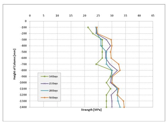
Figure C2: Column C2 – Cardboard Tube, Normal Concrete
