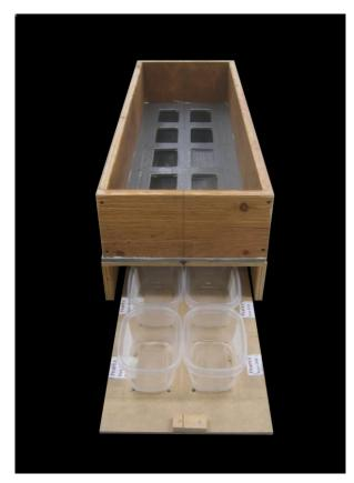
Figure 8: Box made for Box Test using normal concrete
