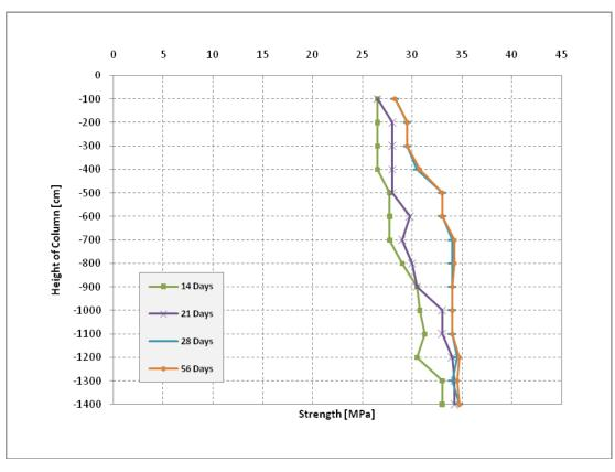
Figure C4: Column C4 – Cardboard Tube, Flyash Concrete
