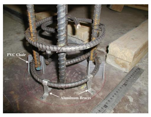
Figure 45: Details of the bottom of the column
