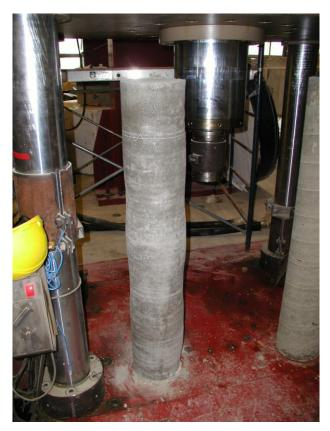
Figure 67: Bulged concrete column
