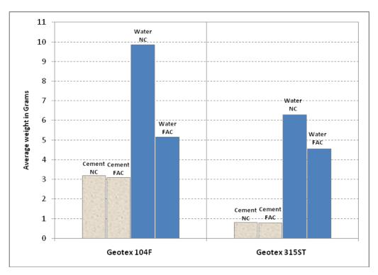
Figure 15: The effect of flyash on the amount of bled water and cementitious material
