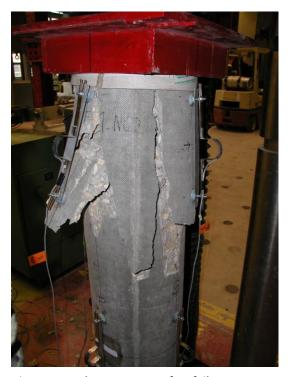
Figure 64: Column FF-NC-2 after failure
