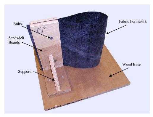
Figure 20: Actual fabric formwork for 152 by 305 mm (6 by 12 in.) concrete cylinders
