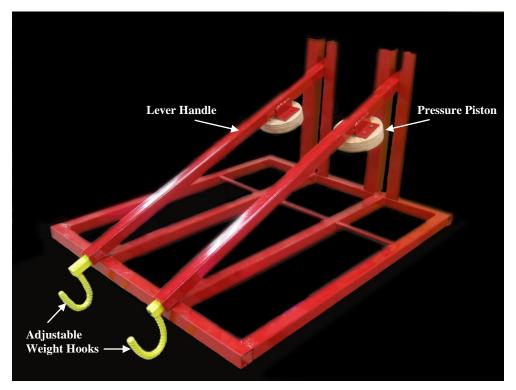
Figure 27: Finished Press machine
