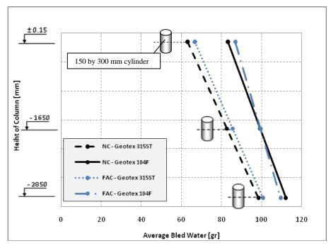
Figure 30: Average water loss through fabric formed cylinders
