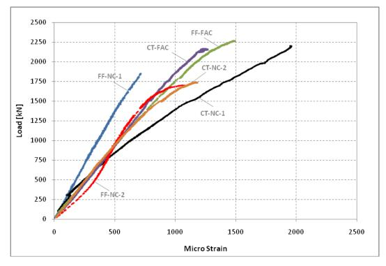
Figure 56: Readings from North pi-gauges at the middle of all columns
