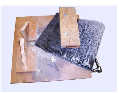
Figure 25: Reusable fabric form parts; the base, sandwich boards, bolts, and the fabric itself
