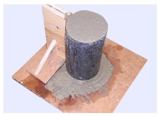
Figure 22: Fabric mold filled with fresh concrete
