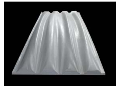
Fig. 9. 2m model funicular shell mold buckled by selective prestressing
