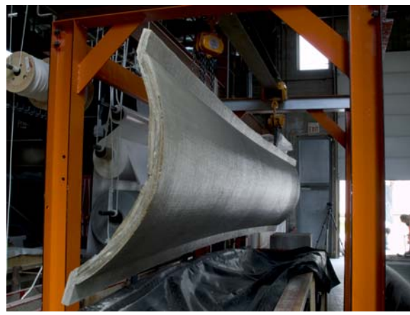
Fig. 2. 3cm thick, 5m long, carbon reinforced shell cast from the fabric mold shown in fig.3
