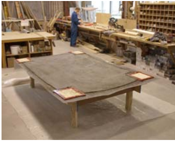
Fig. 4. Test of hanging, fuzzy-backed Fabric, coated with 5mm GFRC
