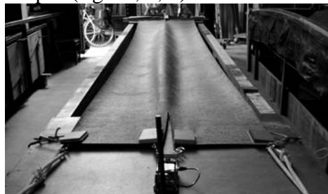
Fig. 8. Flat fabric sheet buckled by selective Pre-stressing, prepared for a 6m shell mold
