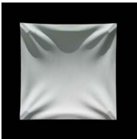
Fig. 7. Corrugations in shell vault along principle stress lines
