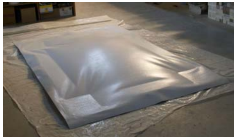
Fig. 5. The fig. 4 funicular mold inverted, showing the plastic-coated release surface
