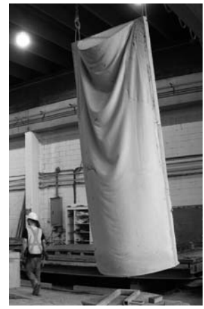
Fig. 3. 4cm thick, thin-shell, fiber-reinforced wall panel
