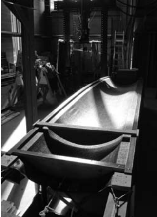
Fig. 1. Flat sheet fabric mold for a double curvature shell
