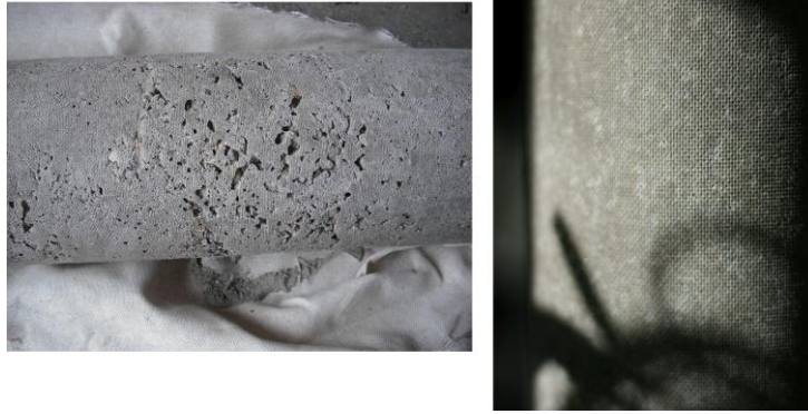
Figure 3: Column 1, w/c ratio = 0.50 Column 2, w/c ratio = 0.55
