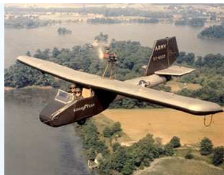
Figure 10 3D fabric layout (Holtmark, 2001) Figure 11 Goodyears Inflatoplane
