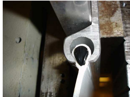
Figures 14 and 15: Illustration aluminium kedder -profile and photo during testing
