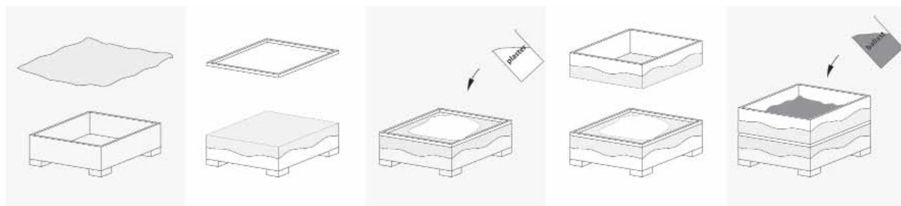
4-4: Process of casting plaster samples
