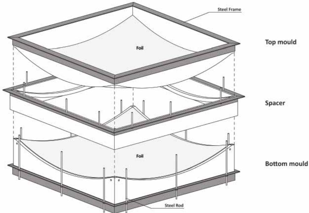
4-11: Exploded view of the mould
