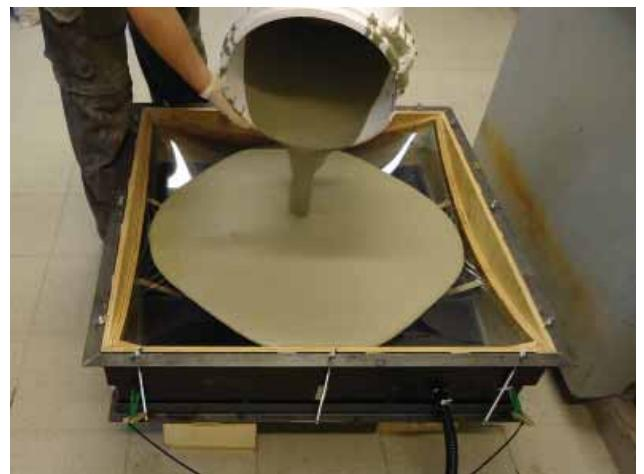
4-36: Grey concrete poured into the mould
