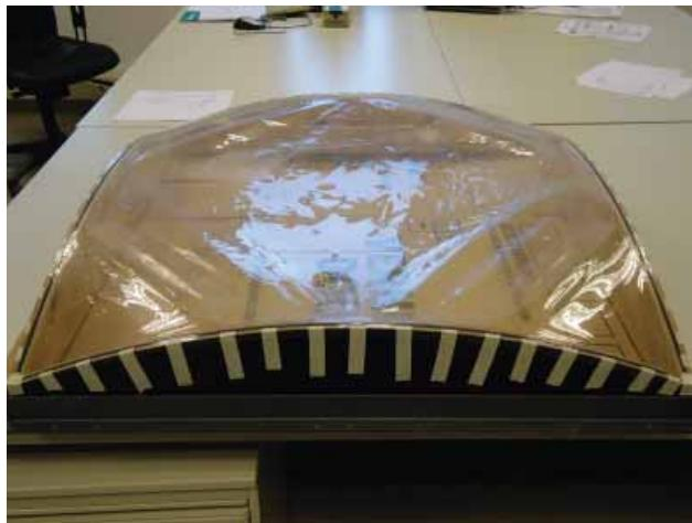
4-34: Plastic deformations in foil (before restretching)
