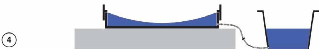
4-18: Process of casting a concrete segment
