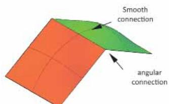
3-23: Connection between flat mould-segments
