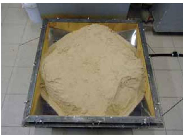
4-22: Top mould is loaded with sand
