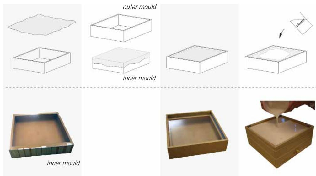
3-6: Process of casting plaster sample
