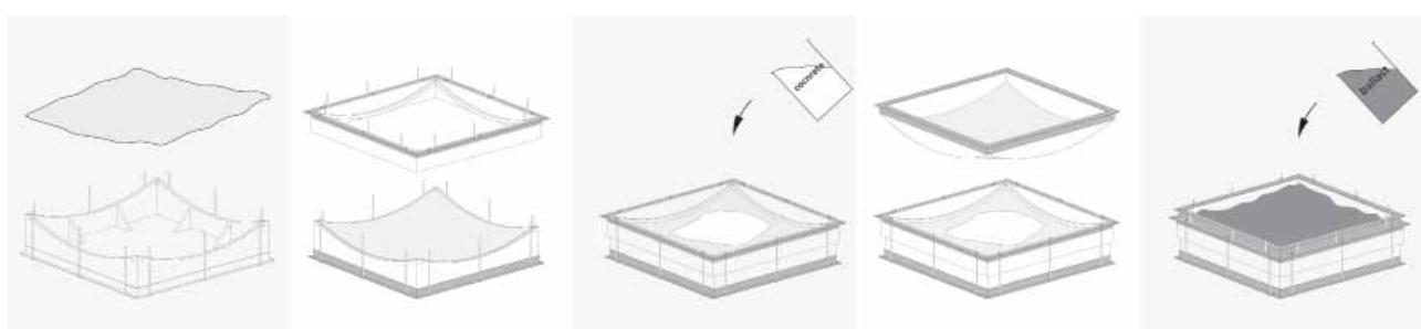
4-14: Process of casting concrete segments
