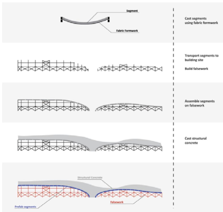
2-18: Building process with prefabricated fabric formwork
