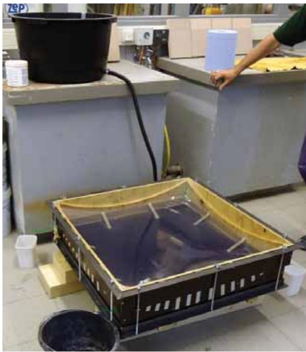
4-19: Filling the bottom mould with water
