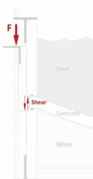
4-13: Shear force in spacer edge
