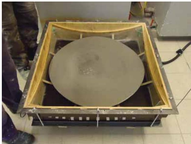
4-27: Wet concrete poured on bottom foil
