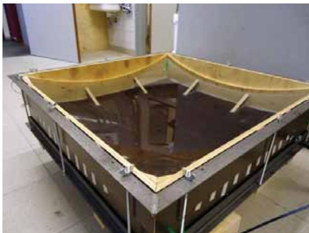
4-20: Bottom mould filled with water
