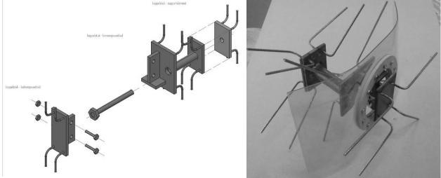
Figure 17: Anchoring the different sections
