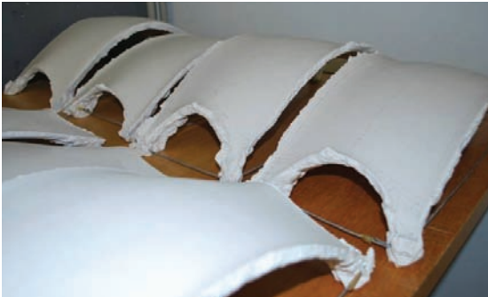
Figure 4: Series of form-finding models for Isler's standard typically 17.75 or 18.6 m wide x 48 m long tennis hall shells. (Photograph: John Chilton)
