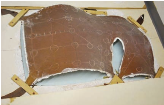
Figure 2: Latex rubber form-finding model for the Sicli SA factory shell in Geneva (Photograph: John Chilton)
