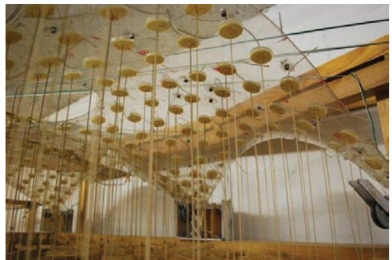
Figure 9: Detail of structural model for the Sicli SA factory, Geneva, 1969. (Photograph: John Chilton)
