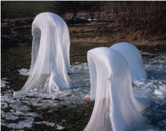
Figure 13: Draped frozen fabric becomes self-supporting in compression once the supporting forms are removed (Photograph: © Heinz Isler Archive)
