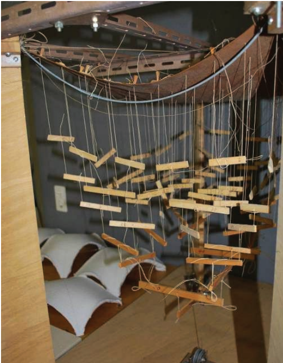
Figure 3: Mechanical form-finding rig for surface similar to the Deitingen Süd motorway service station shells seen in Isler's studio at Lyssachsachsen (Photograph: John Chilton)
