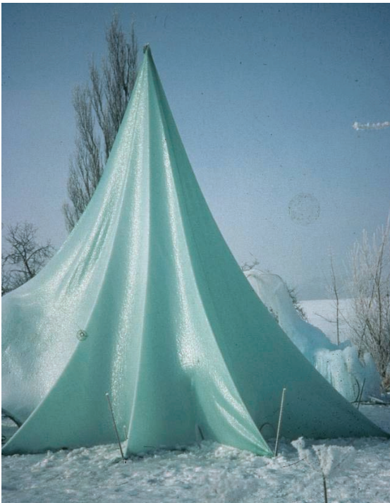
Figure 14: Draped frozen fabric initially supported by a central pole (Photograph: © Heinz Isler Archive)
