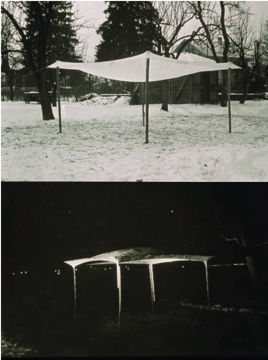
Figure 10: The hanging and inverted membrane shown in Isler's IASS Congress paper, 1959. (Photographs: © Heinz Isler Archive)
