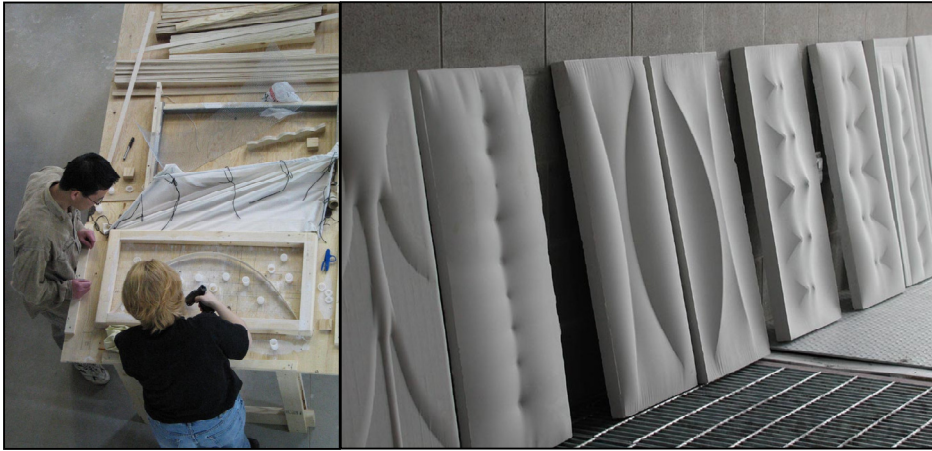
Figure 3: Model formwork and completed plaster casts. (C.A.S.T. photos).
