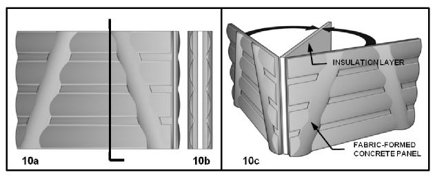
Figure 10. Computer aided design drawing of a fabric-cast wall panel system (Figures by RPS).
