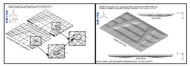
Figure 5. "Form-finding" combined fabric and slurry model (left), resultant panel shape (right) (Figures by RPS).
