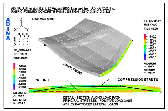
Figure 7. Panel principal stresses under positive loads along diagonal rib (Figures by RPS).
