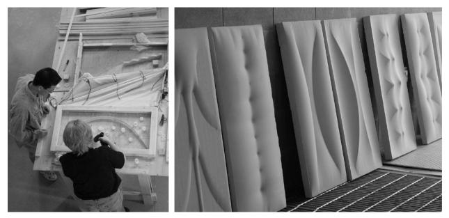
Figure 3. Model formwork and completed plaster cast (C.A.S.T. photos).
