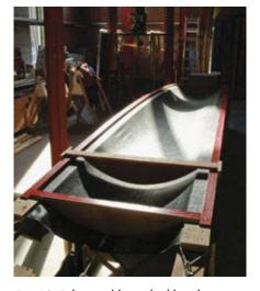
Fig. 19. Fabric mold stretched lengthwise in frame to form double curvature funicular thin-shell vault (C.A.S.T. photo)
