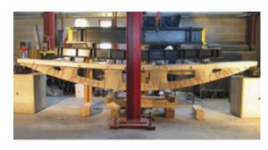
Fig. 13. Testing of variable section concrete truss (C.A.S.T. photo)
