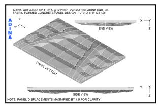
Fig. A2. Final concrete panel shape using FEA.
