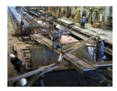
Fig. 15. Step 2- Uniform layer of GFRC is applied (C.A.S.T. photo)
