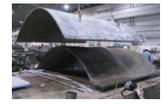
Fig. 17. Step 4 – Thin-shell funicular GFRC vault produced from mold (C.A.S.T. photo)
