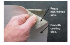
Fig. 18. Fabric for forming rigid molds (C.A.S.T. photo)
